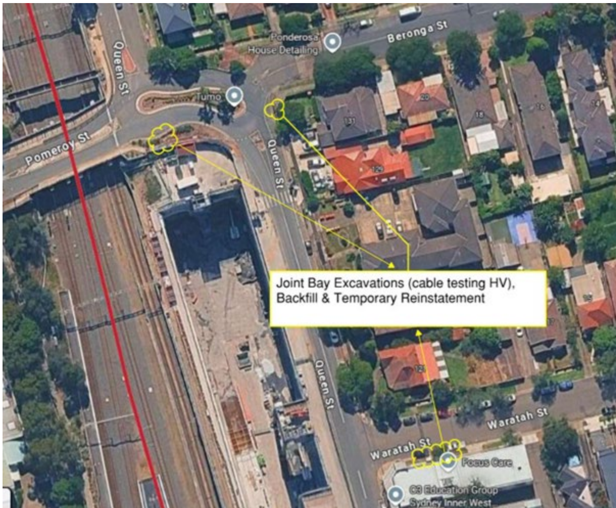
Figure 5-3 Joint Bay Excavations, Backfill and Temporary Restoration Locations
